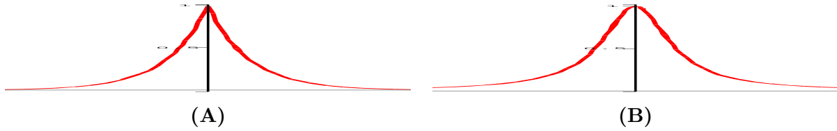
Figure 17.4: (A) The symmetric exponential tail function f(x) = e^{-\alpha|x|} from Example 17.8. (B) The Fourier transform \hat{f}(x) = \frac{a}{\pi(x^2 + a^2)} of the symmetric exponential tail function from Example 17.8.
